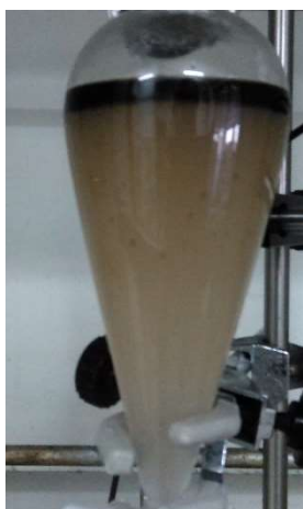
Figure 36. Phase transfer of AuNCs between water and styrene (ME1).
